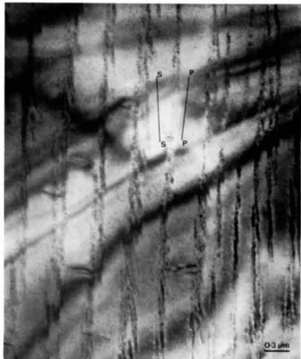
Fig. 15. (a) Diffraction-contrast fringes due to planar faults. Dark field. g = \bar{1}\bar{2}3 . (b) Bright-field ( g = 123 ) micrograph showing planar faults. Note the discontinuous nature of these faults. SS is the trace of shorter segments and PP is the trace of (011).
