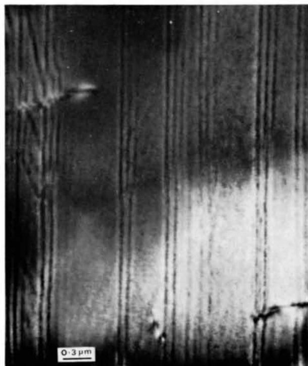
Fig. 15. (a) Diffraction-contrast fringes due to planar faults. Dark field. g = \bar{1}\bar{2}3 . (b) Bright-field ( g = 123 ) micrograph showing planar faults. Note the discontinuous nature of these faults. SS is the trace of shorter segments and PP is the trace of (011).
