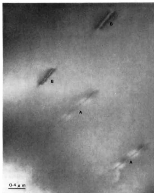
Fig. 10. Dark-field electron micrograph. Dislocations labelled A are out of contrast. g = 02\bar{2} .
